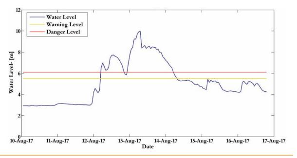
Figure 4.4(b) Water level of Babai River at Chepang station during 2017 flood
