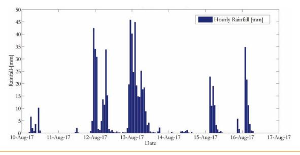
**Figure 4.4(a)** Rainfall recorded at Chepang station during 2017 flood Source: DHM 2017
