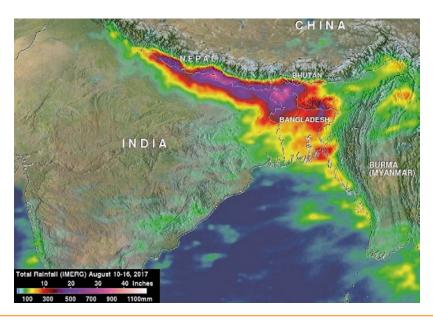
**Figure 1.3** Nepal floods measured by NASA's Integrated Multi-Satellite Retrievals (IMERG) Source: https://pmm.nasa.gov/extreme-weather/deadly-southern-asia-flooding-rainfall-measured-nasas-imerg
